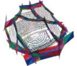
ODEON REFLECTOR COVERAGE 1st ORDER REFLECTIONS
